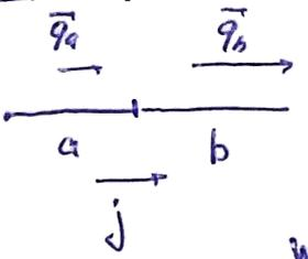
$$W = (\Pi_a - \Pi_b) j \leftarrow \text{heat is released or absorbed at the contact depending on the current direction.}$$
