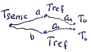
$$\Delta \phi = \int_{T_0}^{T_{ref}} S_a dT + \int_{T_{ref}}^{T_{sens}} S_a dT + \int_{T_{sens}}^{T_{ref}} S_b dT + \int_{T_{ref}}^{T_0} S_b dT = \int_{T_{ref}}^{T_{sens}} (S_a - S_b) \cdot dT$$
